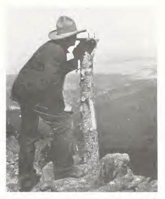
Figure 5. Lookout guard D. W. Edgar sighting fire with alidade and protractor on top of Baldy Mountain (11,200 feet), Apache National Forest, Arizona, 1913 (U. S. Forest Service photo, 15236A).
